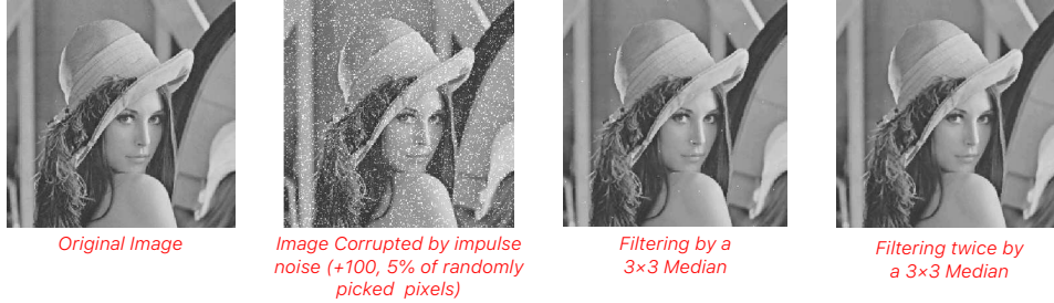
Figure 2.7: Example of median filter application
