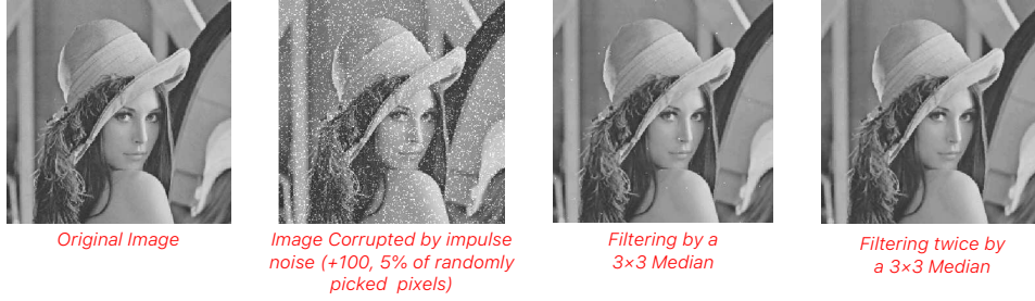
Figure 2.7: Example of median filter application
