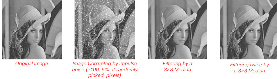
Figure 2.7: Example of median filter application
