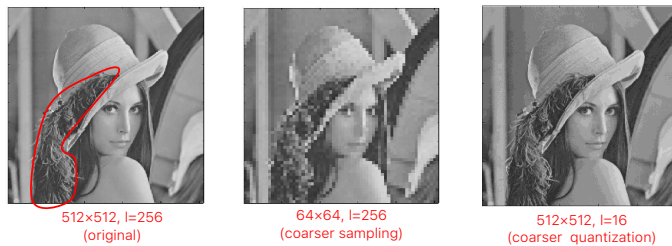
Figure 1.13: Sampling and quantization using fewer bits
