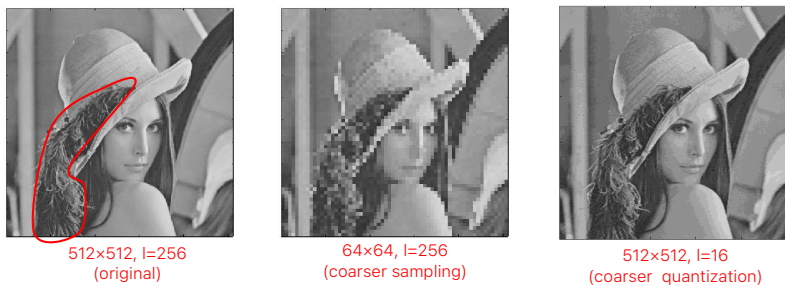
Figure 1.13: Sampling and quantization using fewer bits
