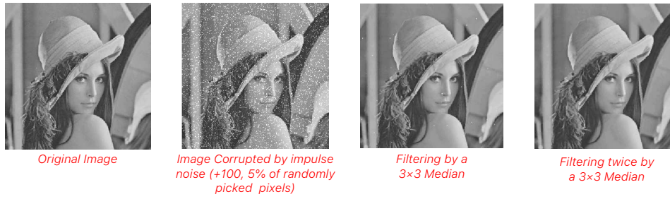
Figure 2.7: Example of median filter application
